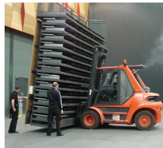
Type M - Mobile. Once closed, units can be specified to be moved via (pictured left to right): a pair of hydraulic trucks, hydraulic trucks with an additional power truck to assist, or fork lift truck.
