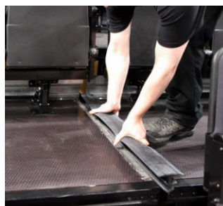
Deck infills - hinged steel, or removable rubber to create joint between two adjacent mobile units.
