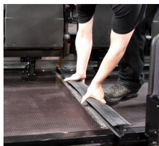
Deck infills - hinged steel, or removable rubber to create join between two adjacent mobile units.
