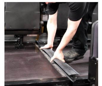
Deck infills - hinged steel, or removable rubber to create join between two adjacent mobile units.
