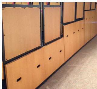
To disguise and prevent access to understructure. Removable panels are available for the side, rear and front of the seating unit (if row 1 is raised) in 16mm MDF with melamine facing, oak finish. Other finishes on request. Removable drapes in fire retardant dimout fabric are also available for the side and rear of the seating unit.
