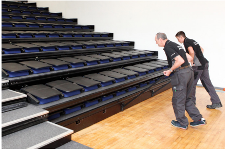
Manual operation via removable pull handles.
